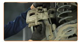
25 Install the brake caliper retaining spring. Use a flat screwdriver.
