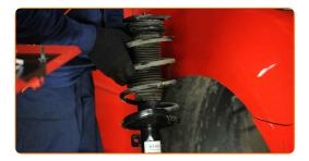
Secure the upper fasteners of the shock strut (3 pieces).
