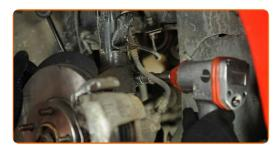
Remove the fastening bolt.
