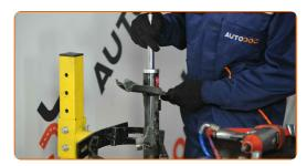
Replacement: suspension strut – Mazda 3 BK. Tip from AUTODOC:
