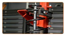
Install the mount, dust boot, and bump stop on a new shock absorber.
