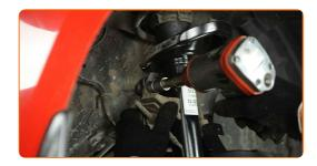
Treat the shock strut fasteners. Treat all joints of the stabiliser link. Use copper grease.
