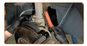
Unscrew the lower fastener connecting the shock strut to the steering knuckle. Use a drive socket #17. Use a ratchet wrench.
