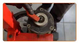
Remove the strut piston rod nut. Use a combination spanner #19. Use HEX No.H6. Use a ratchet wrench.
