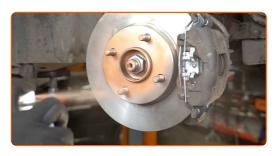
52 Clean the brake disk surface. Use a brake cleaner.
