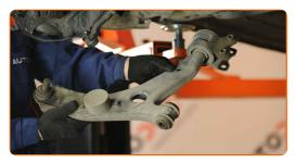
Unscrew the fasteners and remove the bump stop from the front independent suspension lower control arm. Use a drive socket #12. Use a ratchet wrench.
