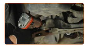
Tighten the rear fastener of the control arm. Use a drive socket #18. Use a torque wrench. Tighten it to 86 nm torque.
