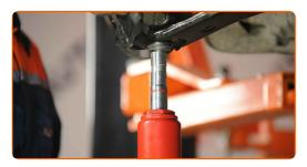
Tighten the front fastener connecting the control arm to the subframe. Use a drive socket #18. Use a torque wrench. Tighten it to 130 nm torque.
