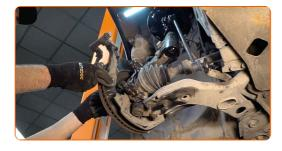
19 Remove the brake disc.
