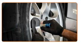
28 Lower the car and working in a cross order, tighten the wheel bolts. Use a torque wrench. Tighten it to 120 Nm torque.
