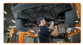
Put a waste oil container with at least 4 l capacity under the drainage hole.
