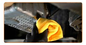
Screw in the new drainage plug and tighten it. Use a drive socket No.19 or ring spanner No.19. Use a torque wrench. Tighten it to 30 nm torque.
