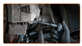
16 Remove the brake caliper.
