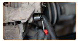
Connect the ABS sensor electric socket. Connect the brake pad wear sensor plug.
