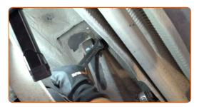
Unscrew the lower fastener of the shock absorber. Use a combination spanner #18. Use a drive socket #18. Use a ratchet wrench.
