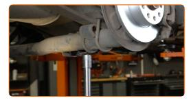
Tighten the lower fastener of the shock absorber. Use a combination spanner #18. Use a drive socket #18. Use a torque wrench. Tighten it to 75 Nm torque.+90°
