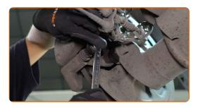
Remove the brake caliper. Use a crowbar.
