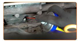
Unscrew the glow plugs. Use the spark plug socket #10. Use a torque wrench.
