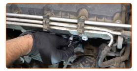
Tighten the glow plugs. Use the spark plug socket #10. Use a torque wrench. Tighten it to 15 nm torque.
