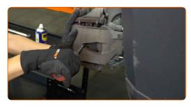
10 Remove the brake caliper.
