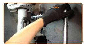
Tighten the fastener connecting the stabilizer link to the stabilizer bar. Use a combination spanner #15. Use a drive socket #19. Use a torque wrench. Tighten it to 60 Nm torque.
