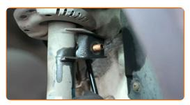
Tighten the fastener connecting the stabilizer link to the shock strut. Use a combination spanner #15. Use a drive socket #19. Use a torque wrench. Tighten it to 60 Nm torque.
