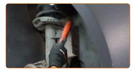
Unscrew the fastener connecting the stabilizer link to the stabilizer bar. Use a combination spanner #18.
