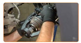
Install and tighten the drive shaft bolt. Use a drive socket #27. Use a ratchet wrench.
