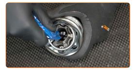
Move the inner race of the new CV joint from side to side to get it ready to work.
