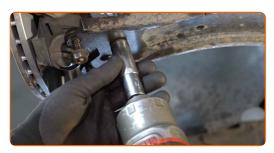
Install and tighten the drive shaft bolt. Use a drive socket #27. Use a ratchet wrench.
