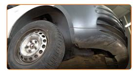
Tighten the bolt connecting the drive shaft to the wheel hub. Use a drive socket #27. Use a torque wrench. Tighten it to 200 Nm torque.+180°
