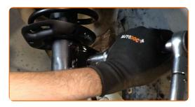
Treat the shock strut fasteners. Treat the fasteners of the ball joint. Treat all joints of the stabiliser link. Use copper grease.
