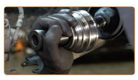
Install the boot on the CV joint.
