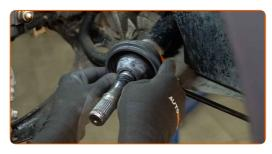
29 Install the CV joint circlip.
