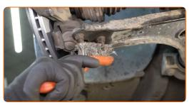
Unscrew the fastener connecting the ball joint to the suspension control arm. Use a drive socket #16. Use a ratchet wrench.
