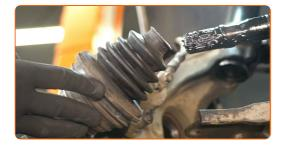
Clean the CV joint mounting seat. Use all-purpose cleaning spray.
