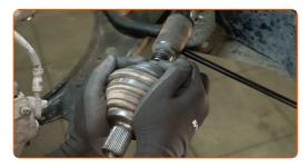
19 Attach the CV joint puller.
