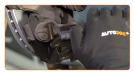
Detach the driveshaft from the steering knuckle.
