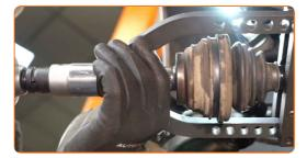
Detach the CV joint. Use a CV joint puller.
