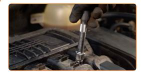
Screw new spark plugs and tighten them. Use the spark plug socket #16. Use a torque wrench. Tighten it to 28 nm torque.
