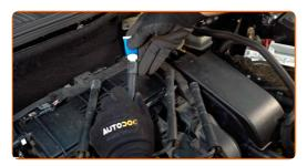
Install the spark plug wire connectors into the spark plug wells. Use round-nose pliers. Make sure you hear a click indicating that it is locked in place.
