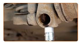
Remove the mounting from under the rear axle beam.
