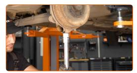
Attach the lower part of the shock absorber.
