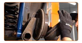
Clean the hub bearing mounting seat. Use all-purpose cleaning spray.
