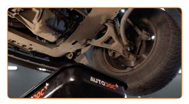
8 Unscrew the drain plug. Use square oil drain plug socket No.8
