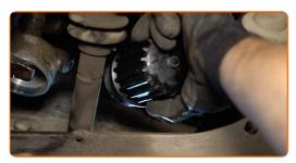
Screw the new filter into its place. Use the 66-6F socket. Use a torque wrench. Tighten it to 25 nm torque.
