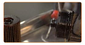
Install new O-rings (2 pieces) and a new oil filter to their mounting seats on the filter cover.
