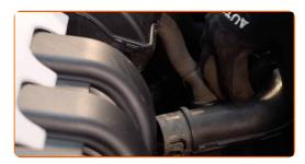
Undo the fastening screws of the air filter cover. Use a drive socket #10. Use a ratchet wrench.
