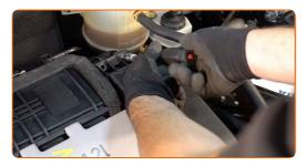
11 Attach the coolant tank hose.
