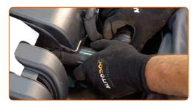
Remove the fender protection cover.
