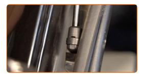
Snap on the circlip connecting the gas strut to the car body.
