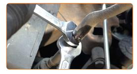
Unscrew the end fastening nut to the steering knuckle. Use a drive socket #16. Use a tap wrench.
