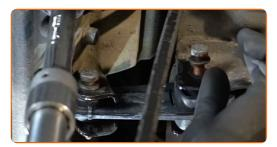
Screw in the fasteners that connect the engine mount to the car body. Use a drive socket #16. Use a ratchet wrench.
