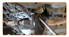
18 Remove the support from under the gearbox.
