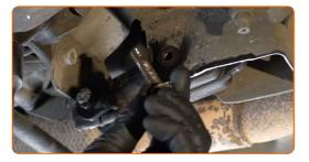
Unscrew the fastener connecting the engine mount to the gearbox housing. Use a drive socket #16. Use a ratchet wrench.
