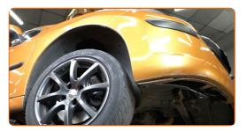
Remove the fender protection cover.
