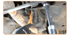
Install the engine mount to its mounting seat.
