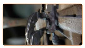
Clean the brake caliper fasteners. Use a wire brush. Use all-purpose cleaning spray.
