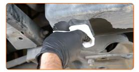
Screw in the new drainage plug and tighten it. Use HEX No.H6. Use a torque wrench. Tighten it to 30 Nm torque.
