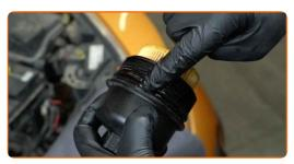
Install a new oil filter housing cover and tighten it. Use a drive socket #27. Use a torque wrench. Tighten it to 25 Nm torque.
