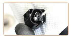
Plug in the ignition coil connector. Make sure you hear a click indicating that it is locked in place.
