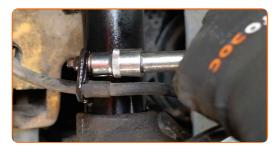
Disconnect the brake hose mounting bracket.
