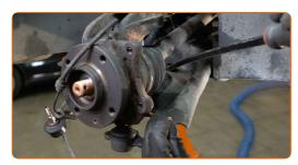
Screw the fasteners of the ball joint. Use a drive socket #16. Use a ratchet wrench.
