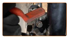
Unscrew the brake hose fastening bracket from the shock strut. Use a combination spanner #13.
