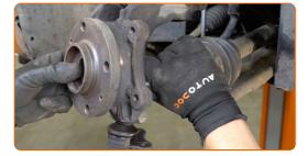
Disconnect the steering knuckle from the shock absorber strut. Use a hammer.
