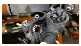
Place the steering knuckle assembled with the wheel hub in a vice.
