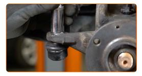
Tighten the fasteners connecting the ball joint to the control arm. Use a drive socket #16. Use a torque wrench. Tighten it to 60 Nm torque.
