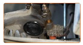
Unscrew the lower fastener connecting the shock strut to the steering knuckle. Use a drive socket #16. Use a ratchet wrench.
