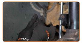
Clean the mounting seats of the tie rod end. Use a wire brush. Use WD-40 spray.
