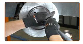
24 Remove the brake disc.
