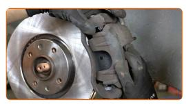
Tighten the brake caliper bracket. Use Torx T55. Use a torque wrench. Tighten it to 105 Nm torque.
