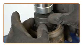
Clean the hub bearing mounting seat. Use all-purpose cleaning spray. Use WD-40 spray.
