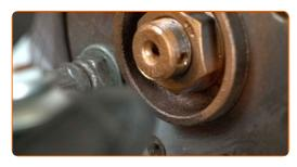
Install the CV axle nut cotter pin. Use a crowbar.
