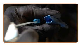
Attach the ABS sensor connector.
