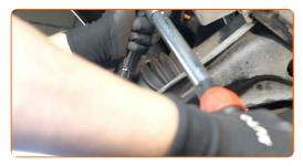
81 Secure the brake hose bracket.
