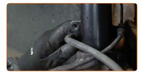
Tighten the fastener connecting the brake hose bracket to the suspension strut. Use a drive socket #13. Use a torque wrench. Tighten it to 10 nm torque.
