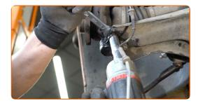
Disconnect the ball joint from the arm. Use a crowbar.
