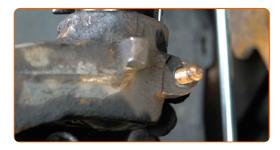
Screw in the fastener that connects the shock strut to the steering knuckle. Use a drive socket #16. Use a ratchet wrench.
