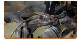
Fix the shock absorber strut on the steering knuckle.
