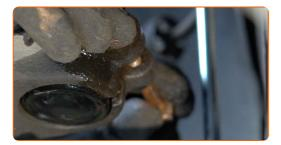
Detach the driveshaft from the steering knuckle.
