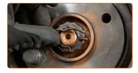
Treat all joints of the stabiliser link. Treat all joints of the arm. Use copper grease.
