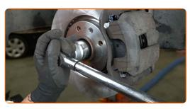
Treat the CV axle fastener. Use copper grease.
