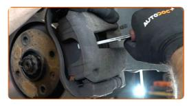
10 Remove the brake caliper.
