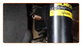
Tighten the fastener connecting the stabilizer link to the shock strut. Use a drive socket #17. Use a torque wrench. Tighten it to 43 Nm torque.
