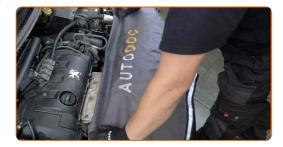
Disconnect the air intake pipe fastening. Use a drive socket #10. Use a ratchet wrench.
