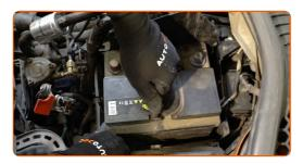
Remove the electronic control unit.
