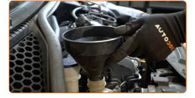
Pour coolant in the coolant reservoir.
