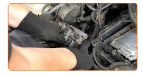
Clean the thermostat housing mounting seat. Use a seal scraper. Use all-purpose cleaning spray.
