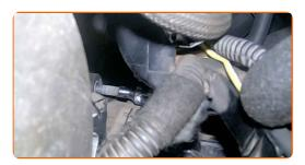
Detach the clip of the upper coolant hose. Use round-nose pliers.
