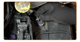
Screw in the fasteners of the battery terminals. Use a combination spanner #8.
