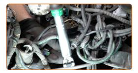
Tighten the thermostat housing mounting stud. Use a drive socket #E5. Use a torque wrench. Tighten it to 11 nm torque.
