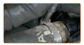
Treat the engine wiring harness connectors. Use electronic spray.
