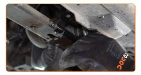
Attach the clamp of the lower coolant pipe. Use a combination spanner #7.
