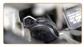
Tighten the thermostat housing fasteners. Use a drive socket #8. Use a drive socket #10. Use a torque wrench. Tighten it to 13 nm torque.
