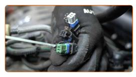
Attach the engine wiring harness connectors.
