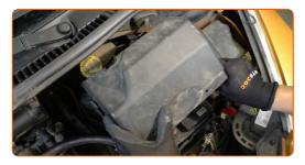
6 Unscrew the fasteners of the car battery terminals. Use a combination spanner #8.
