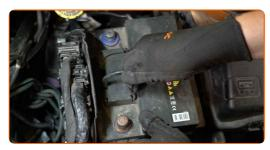
Attach the terminals to the battery.
