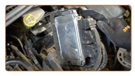
11 Remove the engine wiring harness cover.
