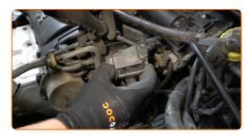
Detach the engine wiring harness connectors. Use a flat screwdriver.
