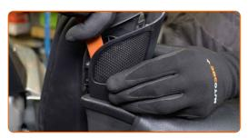
Unscrew the fasteners of the wing mirror trim panel. Use Torx T25.
