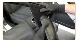
Tighten the screws of the wing mirror. Use Torx T25. Use a drive socket #10. Use a torque wrench. Tighten it to 5 Nm torque.
