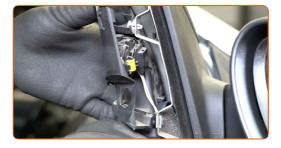
Screw in the fasteners of the wing mirror trim panel. Use Torx T25.
