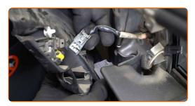
Remove the wing mirror screws. Use Torx T25. Use a drive socket #10. Use a ratchet wrench.
