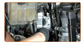
Tighten the engine mount fastening bolts. Use a drive socket #E11. Use a torque wrench. Tighten it to 32 Nm torque.
