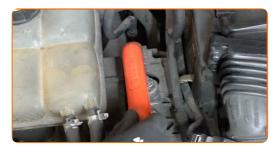
Unscrew the upper fastener of the engine mount. Use a drive socket #16. Use a ratchet wrench.
