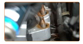
Tighten the upper fastener of the engine mount. Use a drive socket #16. Use a torque wrench. Tighten it to 55 Nm torque.
