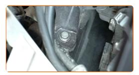
Unscrew the fasteners that connect the engine mount to the car body. Use a drive socket #18. Use a ratchet wrench.
