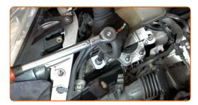
Treat the engine mount fasteners. Use copper grease.
