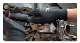
Clean the brake caliper bracket fasteners. Use a wire brush. Use all-purpose cleaning spray.
