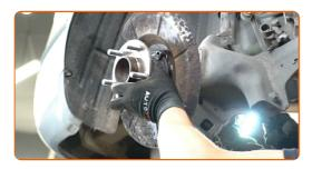
Remove the brake disc baffle plate.
