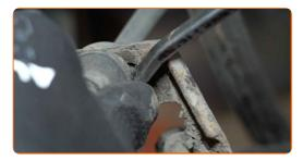
Remove the brake caliper together with its bracket. Use a crowbar.
