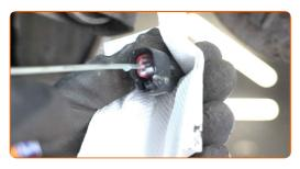
Attach the ABS sensor connector.
