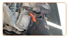
Unscrew the caliper bracket fastening. Use a combination spanner #13.
