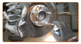
28 Install the brake disc.
