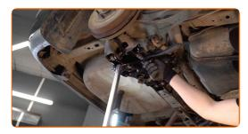
Tighten the shock absorber mount fasteners. Use a drive socket #10. Use a torque wrench. Tighten it to 25 Nm torque.
