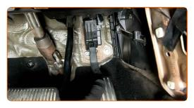
Return the accelerator pedal to its initial position and screw in its fastener. Use a drive socket #10. Use a ratchet wrench.
