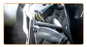
5 Detach the accelerator pedal connector.
