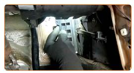
Screw in the fasteners of the cabin filter housing cover. Use a drive socket #8. Use a ratchet wrench.
