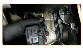
Reinstall the accelerator pedal.
