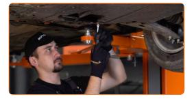
Remove the oil pan cover. Use a drive socket #10. Use a flat screwdriver. Use a ratchet wrench.
