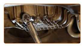
Reinstall the oil pan lower cover. Tighten the fasteners of the oil pan lower cover. Use a drive socket #10. Use a ratchet wrench.
