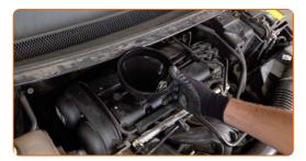
Pour oil into the engine through the filler. Required amount of oil: 3.7 L.
