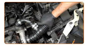
Attach the air inlet pipe to the turbocharger.
