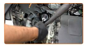
Remove the microfibre cloth from the turbocharger impeller. Remove the microfibre cloth from the PCV valve hole.
