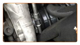
Attach the mass air flow sensor connector.
