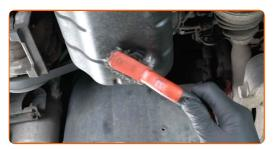
Unscrew the drain plug. Use a drive socket #21. Use a ratchet wrench.
