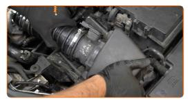
Cover the turbocharger impeller with a microfibre cloth to prevent dirt and foreign objects getting into the system.
