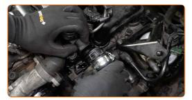
Detach the air inlet pipe from the turbocharger.
