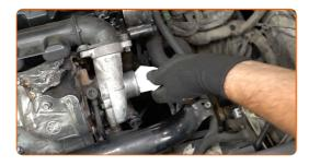
Install the air filter housing and fasten it.
