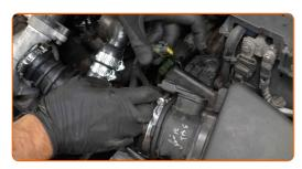
Remove the air filter housing.
