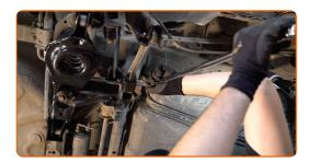
Unscrew the fastener connecting the control arm to the rear knuckle. Use a drive socket #15. Use a ratchet wrench. Remove the fastening bolt.
