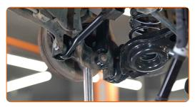
Tighten the arm fastening to the beam. Use a drive socket #15. Use a torque wrench. Tighten it to 115 Nm torque.
