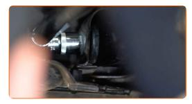
Tighten the rear fastener connecting the arm to the body subframe. Use a drive socket #15. Use a torque wrench. Tighten it to 115 nm torque.
