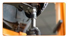
20 Install the fastening nut of the ball joint.
