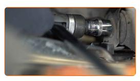
Remove the front fastener of the control arm. Use a crowbar. Use a hammer.
