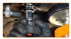
Screw the front arm fastener. Use a drive socket #18. Use a torque wrench. Tighten it to 175 nm torque.
