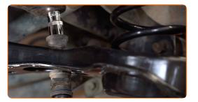
Tighten the lower fastener of the shock absorber. Use a drive socket #16. Use a torque wrench. Tighten it to 103 Nm torque.
