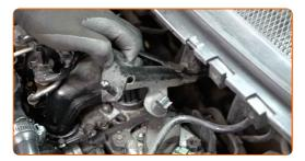
Unscrew the fuel filter bracket. Use a drive socket #E11. Use a ratchet wrench.
