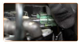
16 Install the fuel filter fastening bracket.
