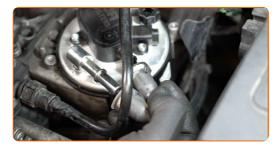
Tighten the fuel filter fasteners. Use a drive socket #E11. Use a torque wrench. Tighten it to 8 Nm torque.
