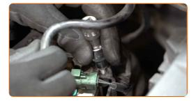
Detach the fuel pressure sensor connector. Use a flat screwdriver.
