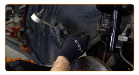
11 Install a new rod, tighten the fasteners.
