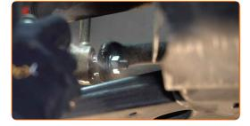
Unscrew the fastener connecting the stabilizer link to the stabilizer bar. Use a combination spanner #15.
