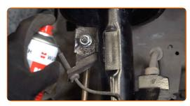
Unscrew the fastener connecting the stabilizer link to the shock strut. Use a drive socket #15. Use a ratchet wrench.
