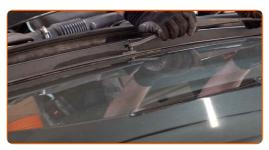
Tighten the fasteners of the wiper arms. Use a drive socket #15. Use a torque wrench. Tighten it to 10 Nm torque.
