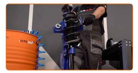
Remove the assembled shock strut.
