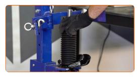
Install the spring on the shock absorber.
