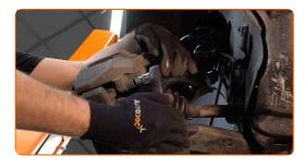
11 Remove the brake caliper.
