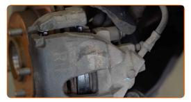
Install the brake caliper retaining spring.
