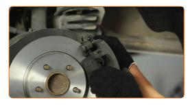
Clean the brake caliper guide pins.
