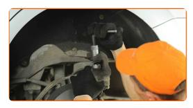
Install the brake caliper and fix it.
