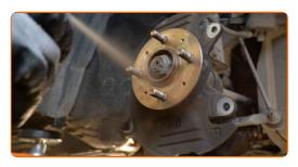
20 Install the brake disc.
