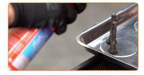
Treat the brake caliper guide pins. Use the brake caliper guide pin grease.
