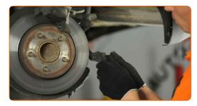
18 Remove the brake disc.
