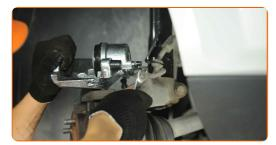
Remove the brake hose clamp.
