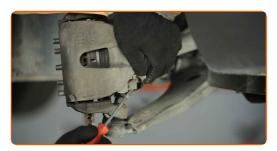
Clean the area where the brake hose is connected to the caliper, and the guide pins area. Use a brake cleaner.
