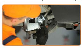
Clean the brake caliper surface.
