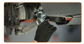
Clean the brake caliper guide pins.
