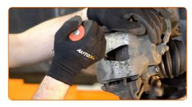
Remove the brake caliper.
