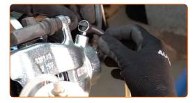
Undo the brake bleeder screw. Use a combination spanner #9.
