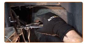
Loosen the brake hose fastening. Use a flare nut spanner #14.
