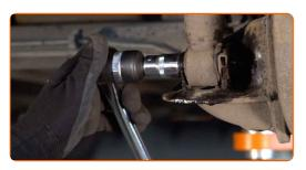
Remove the fastening bolt.
