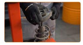
Release the coil spring.
