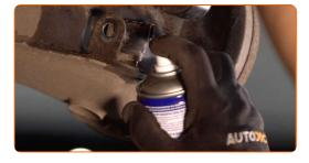
Attach the bottom part of the shock strut.
