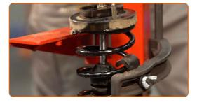
Remove the assembled shock strut.
