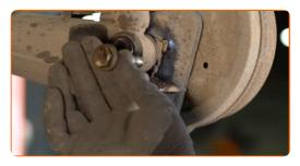
Detach the bottom part of the shock strut.
