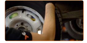
Clean the shock strut fasteners. Use a wire brush. Use WD-40 spray.
