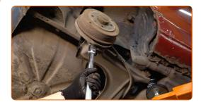
Tighten the lower fastening of the shock absorber. Use a drive socket #18. Use a torque wrench. Tighten it to 95 Nm torque.
