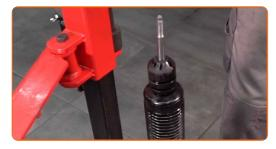
Install the spring on the shock absorber.
