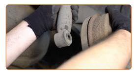
Unscrew the upper fastening of the shock absorber strut. Use a drive socket #13.
