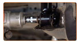
36 Support the rear suspension beam. Use a hydraulic transmission jack.
