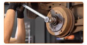
10 Remove the brake drum.
