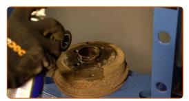
Press a new bearing into the wheel hub. Use a bush and bearing driver set.
