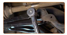
Tighten the ball joint fastener. Use a combination spanner #16. Use a drive socket #16. Use a torque wrench. Tighten it to 62 Nm torque.
