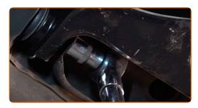
Tighten the front fastener connecting the control arm to the subframe. Use a combination spanner #18. Use a drive socket #18. Use a torque wrench. Tighten it to 115 Nm torque.
