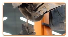
Release the fastener that connects the control arm ball joint to the steering knuckle. Use a flat metal-working chisel. Use a hammer.
