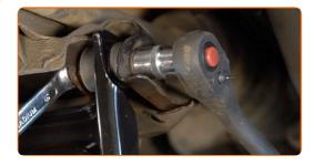
Connect the lower arm to the steering knuckle.
