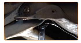
Unscrew the rear arm fastener. Use a combination spanner #19. Use a drive socket #19. Use a tap wrench.
