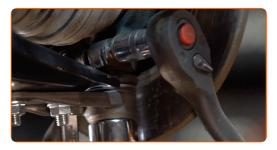
Screw the rear fastener connecting the control arm to the subframe. Use a combination spanner #19. Use a drive socket #19. Use a tap wrench.
