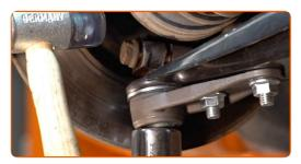
Screw the fasteners of the ball joint. Use a drive socket #16. Use a combination spanner #16.
