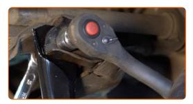
Screw the front arm fastener. Use a combination spanner #18. Use a drive socket #18. Use a tap wrench.
