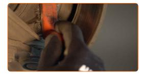
Unscrew the fastener connecting the ball joint to the suspension control arm. Use a combination spanner #16. Use a drive socket #16.
