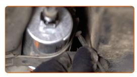
Clean the fasteners of the fuel supply lines. Use all-purpose cleaning spray.
