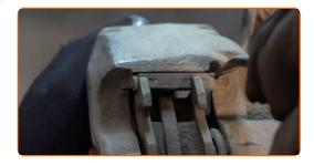
9 Remove the retainer of the brake pads.
