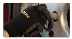
Lower the car and working in a cross order, tighten the wheel bolts. Use a torque wrench. Tighten it to 90 Nm torque.
