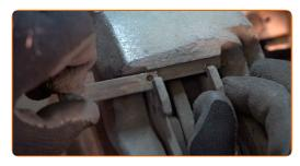
10 Remove the brake pads.
