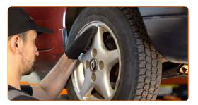
Replacement: brake pads – Renault Twingo C06. Tip from AUTODOC experts:
